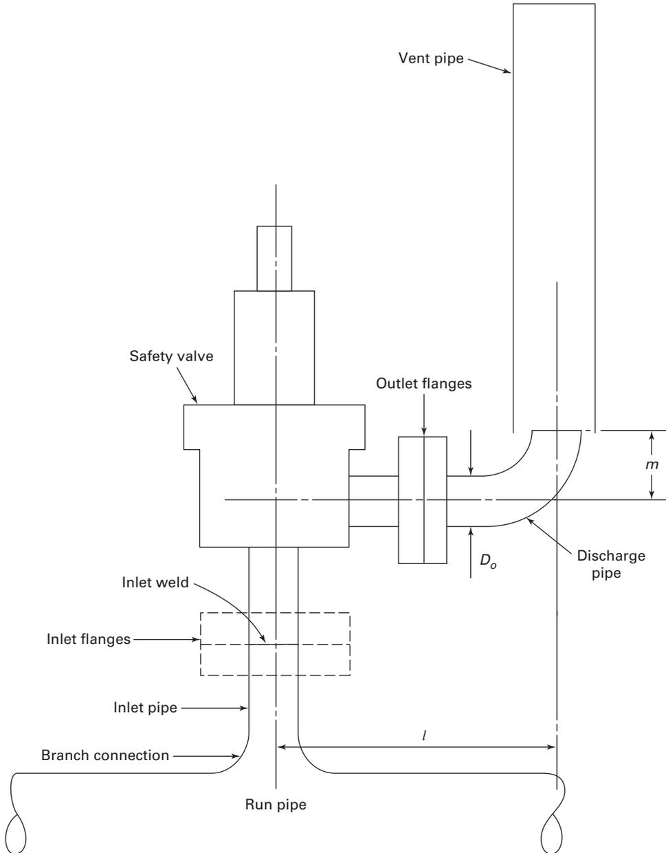
Fig. II-1-2(B) Safety Valve Installation (Closed Discharge System)
