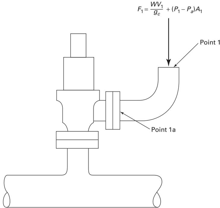
(A.2) Determine the velocity,  $V_1$ , that exists at the discharge elbow outlet (Fig. II-2-1).
