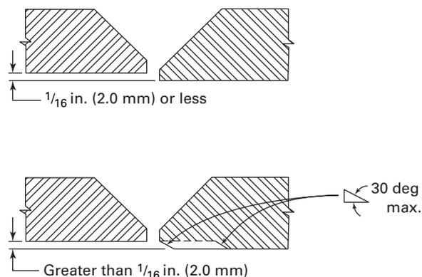
may remain on the flame cut surface is not considered to be detrimental oxidation.
