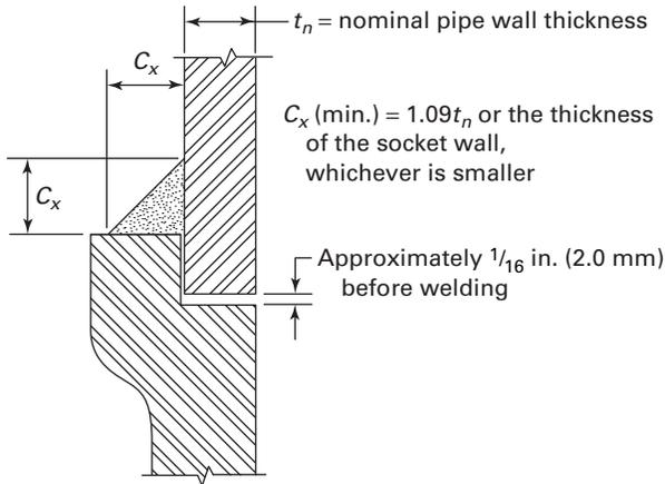
**Fig. 127.4.8(B) Typical Welded Branch Connection With Additional Reinforcement**
