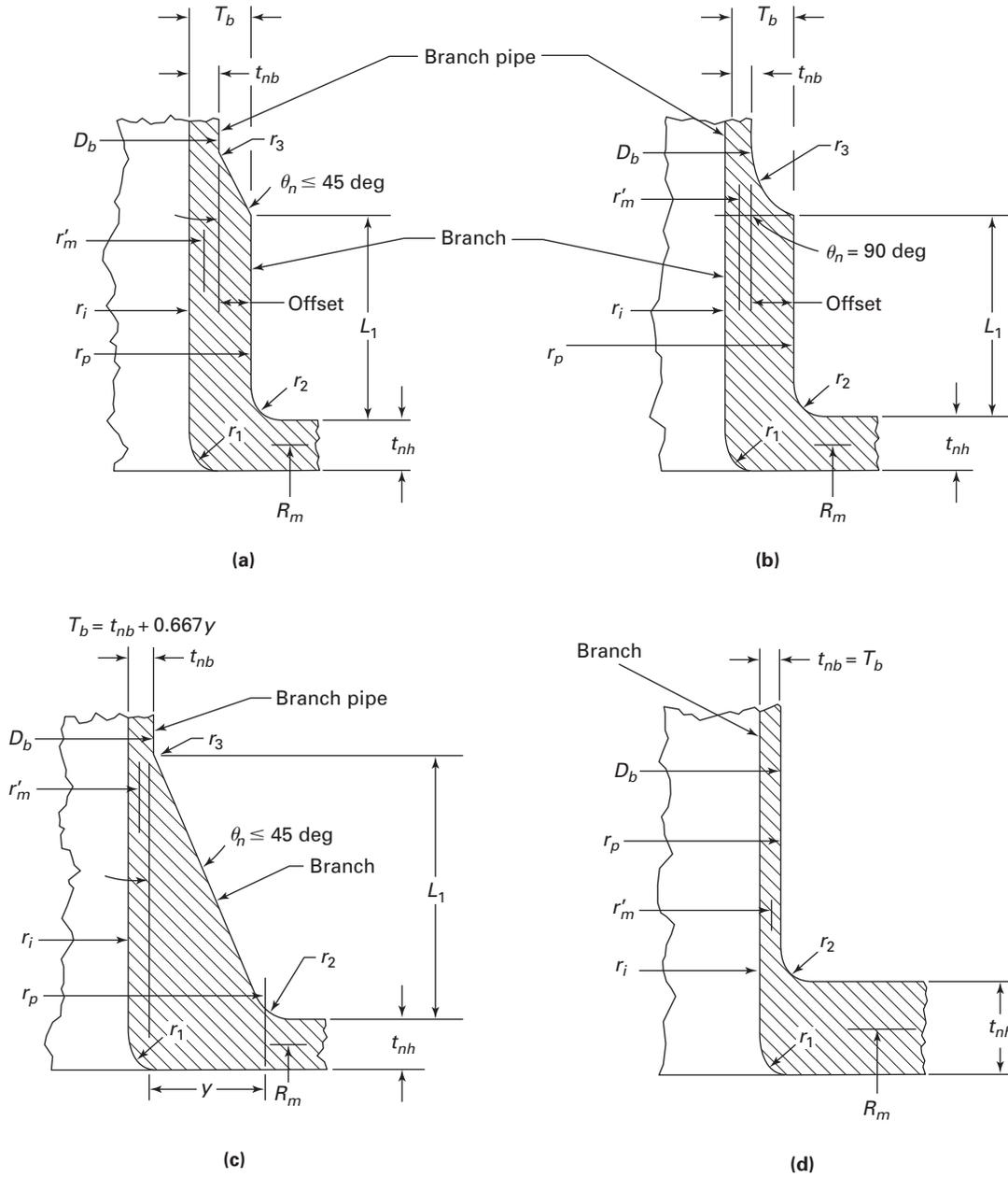
$D_b$  = outside diameter of branch pipe, in. (mm)
