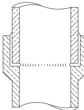
(A.2) *Procedure.* Joints shall be made in accordance with a qualified BPS. ASTM D 2855 provides a suitable basis for such a procedure. Solvent cements for PVC, CPVC, and ABS shall conform to ASTM D 2564, D 2846, and D 2235, respectively. Cement shall be applied to both joint surfaces. The amount of cement shall be sufficient to produce a small continuous fillet of cement at the outer limits of the joints. See Fig. III-5.1.3(A).
