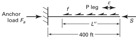
(B) Calculate the load,  $S$ , at the expansion joint.
