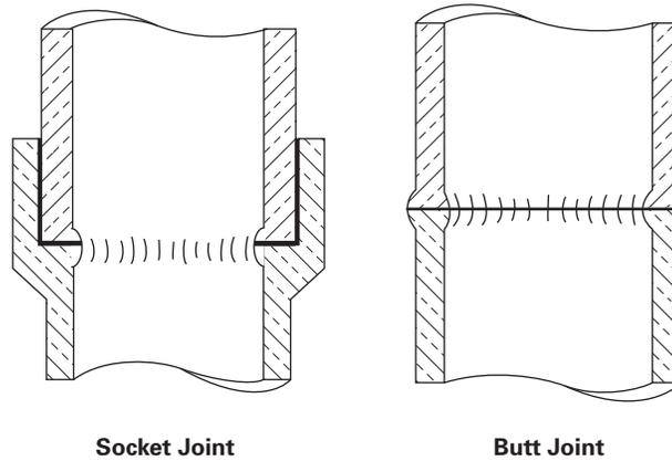
**Fig. III-5.1.3(C) Thermoplastic Electrofusion Joints**
