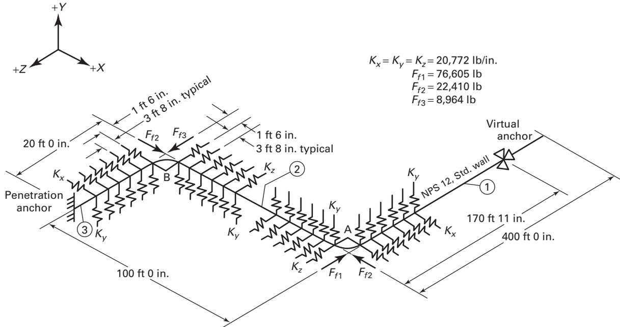
Fig. VII-6.6 Example Plan of Element 1 as a Category D Element
