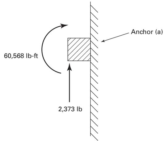
Net imbalance on the vent pipe in the vertical direction is
