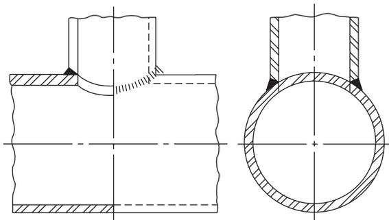
**Fig. 127.4.8(D) Some Acceptable Types of Welded Branch Attachment Details Showing Minimum Acceptable Welds**
