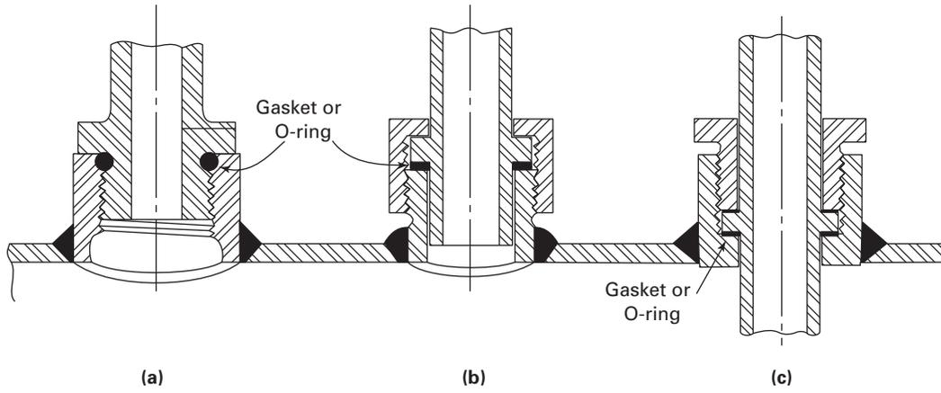
GENERAL NOTE: Threads are ASME B1.1 straight threads.
